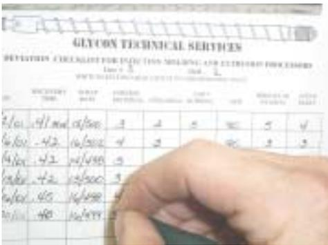
**Fig 1.** Processors should create a form like this one to note important process data, as well as significant part-quality anomalies such as burning, streaking or sticking.
