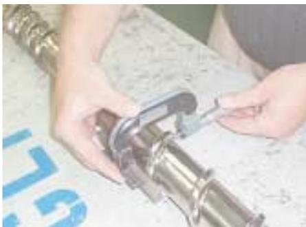
**Fig 2.** Use a flight micrometer or gage block to measure the flight diameter at every turn. Record these readings every six to twelve months to track the progress of wear on the screw.
